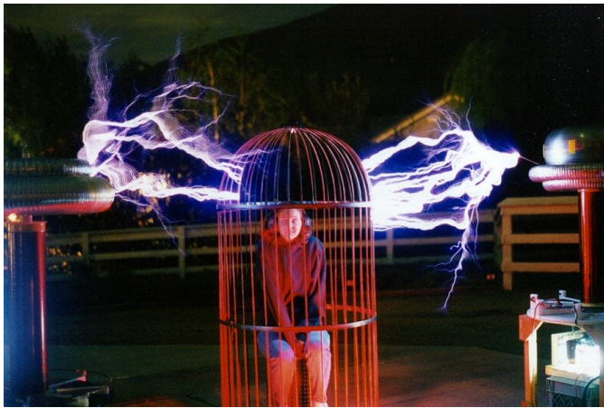
Figure 10. A Faraday Cage protects the contents of the cage from external electrical shocks [16].
